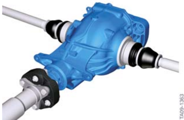
F12 Lightweight construction, rear axle final drive
